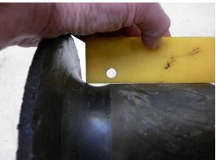
Wear is 2 – 4 mm, the roll is still good. Normally maintenance, inspection on rope. To change the roll is not necessary, do not create unnecessary cost!
