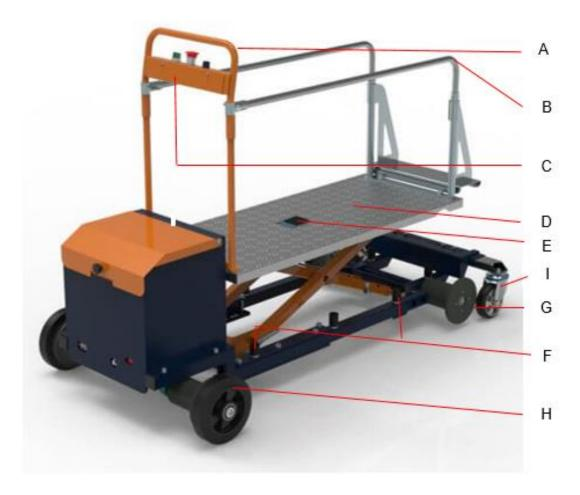
Figure 1: Principal components of the Leaf picking cart
