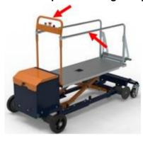
Always use both hands in marked places so that there can never be crushed. When adjusting upwards, a click will be heard at each locking position. If the required height has been attained, carefully allow the platform to drop until it is secured.
