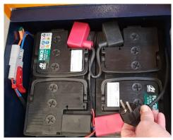
Charge the batteries according to the status of the battery condition meter when they have between 50% and 20% remaining capacity, but try to do this as often as possible when the status is around 20% in accordance with the following recommendations.
