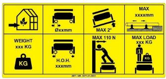
Suitable for the pipe diameter stated with minimum thickness Suitable for the centre-to-centre pipe rail system measurement Maximum sideways manual force in Newtons (kg x10) Maximum total load in kg (maximum 1x person + moveable load) Maximum tilted position 2° Maximum support distance 1250 mm Only to be used indoors (in greenhouse) Mass of the machine in kg
