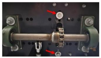
Figure 6: Unscrewing/tightening the motor bolt
