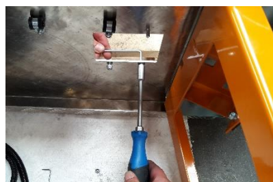
Take a platform (Package B), lay it on a piece of cardboard and unscrew the bolts.
