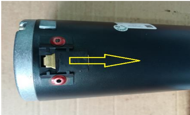
Figures 5b & c: Clean and inspect the carbon brushes
