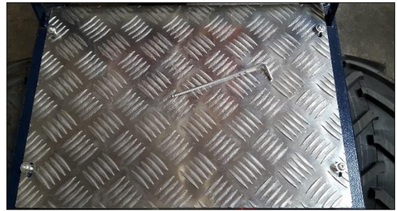
Figure 7: Dismantle the checker plate
