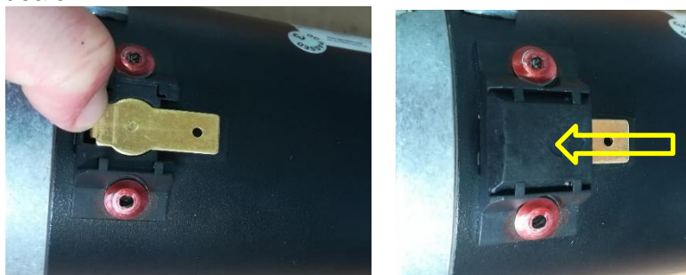
Figures 5d & e: Mounting the carbon brushes
