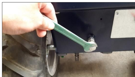
Figure 10: Tension the chain
