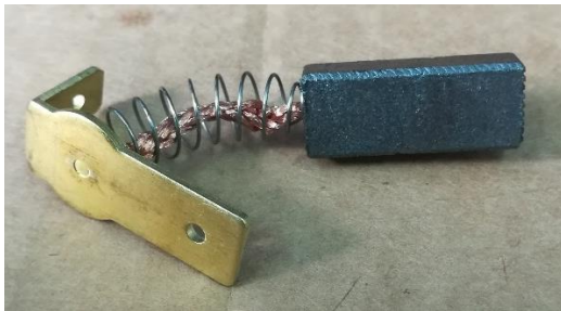
Figure 5d: Inspecting the carbon brushes
