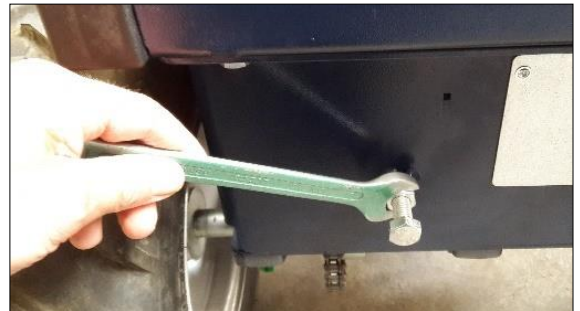
Figure 9: Loosen/tighten the locking nut
