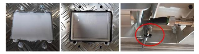
**Step 4**Disconnect the wires from the platform. Cut the fastons off the wires like the picture below.
