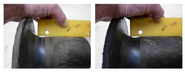
Wear is 2 – 4 mm, the roll is still good. Normally maintenance, inspection on rope. To change the roll is not necessary, do not create unnecessary cost!
