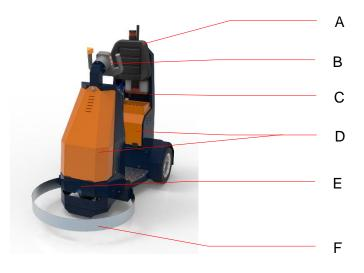
Figure 1: Principal components of the BeTrac 1 AGV
