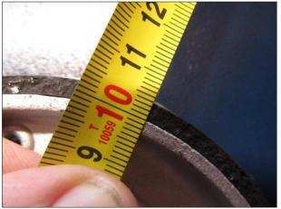
Figure 11: Measure brake shoe lining
