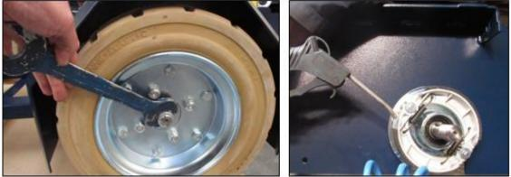
Figure 11: Disassemble wheels
