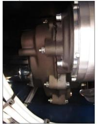
Remove the "towbar panel" by loosening the 4 M10 bolts, behind this panel is the drive motor with differential. Check visually if there is no oil leakage. If the leakage is very small, this can be cleaned with a cloth, do this inspection again after one month to check whether the leakage continues. If there is a leak, consult your dealer.
