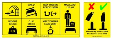
Only to be used indoors Own mass in kg Maximum tilted position 2° Suitable for the centre-to-centre pipe rail system measurement Maximum towing force in Newton Maximum towbar load in Newton Maximum total load in kg (maximum 1x person)
