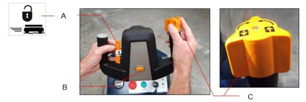
Figure 3: Steering control of the BeTrac 1 AGV
