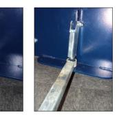
Figure 10: The towing hook locking pin
